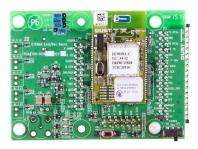
SmartMesh WirelessHART networks are populated by motes, the nodes on the network. Based on the Dust® break-through Eterna® technology, the motes are ultralow power, extending battery life to years and many times that of alternative products. In addition to extra long battery life, the motes feature an advanced array of features.
