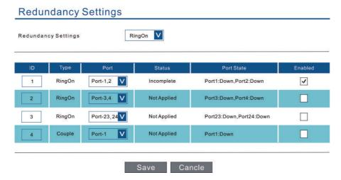
In Redundancy Setting, you can select from Disable, RingON, and RSTP.
