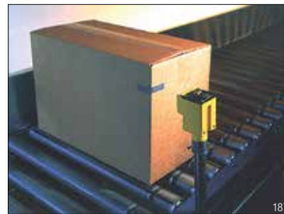
3M™ Retroreflective Materials make it easy to design sensing systems based on simple, inexpensive photoelectric sensors. They increase readability, range and accuracy with greater control.
